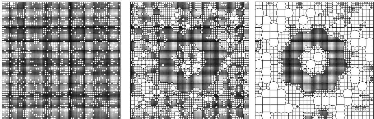
Obr. 3. *On the left: the initial grid (12 658 elements). In the middle: the grid in the 4th scale step (9835). On the right: the final grid (the 10<sup>th</sup> time step with 4615 elements).*
