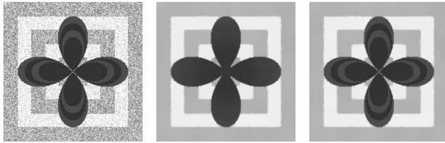
Fig. 1. Restoration of the noisy image (left, 200x200 pixels) by anisotropic diffusion (middle) in comparison with slowed anisotropic diffusion (right); \beta(x, s) = 0 for s \in [0, 0.5] , \beta(x, s) = s for s \in (0.5, 1] .
