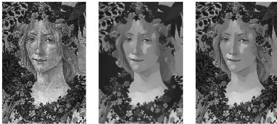
Fig. 2. Restoration of the real image (left, 570x350 pixels) by anisotropic diffusion (middle) in comparison with slowed anisotropic diffusion (right); \beta(x, s) = 0 for s \in [0, 0.39] , \beta(x, s) = s for s \in (0.39, 1] .
