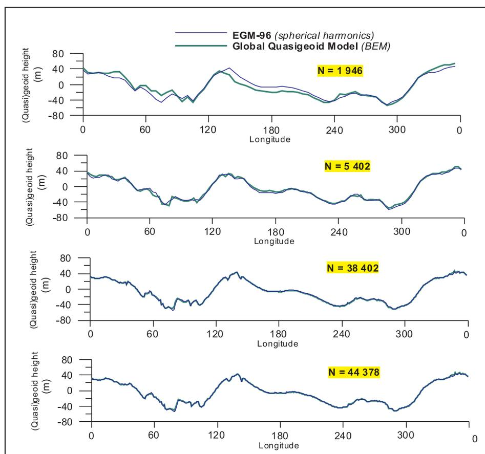
Fig. 5. Comparison with EGM-96 (profiles along the parallel of latitude N 30°).
