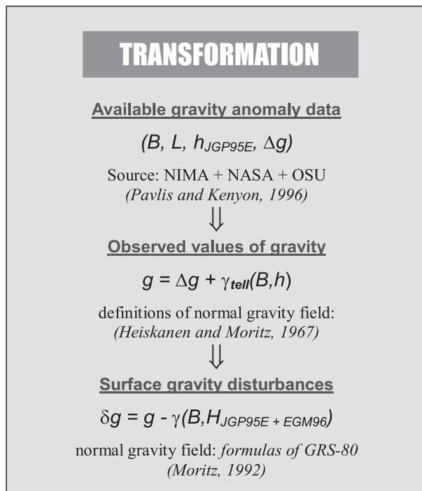
Fig. 2. Surface gravity disturbances generated from the available gravity anomalies.
