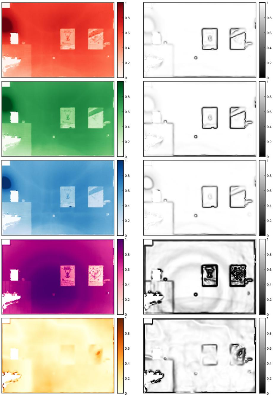
**Fig. 15** Left column: Bitmap images generated from the channels R, G, B, I, D of the point cloud. Right column: Corresponding edge detector functions
