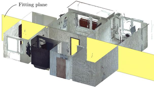
**Fig. 1** Primary segmentation of an apartment scanned by TLS. A planar subset corresponding to a wall was segmented
