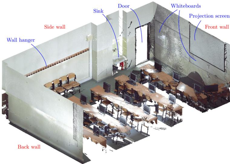
**Fig. 20** Point cloud of the classroom B306 at the Faculty of Civil Engineering of the Slovak University of Technology in Bratislava (ceiling and one wall removed)
