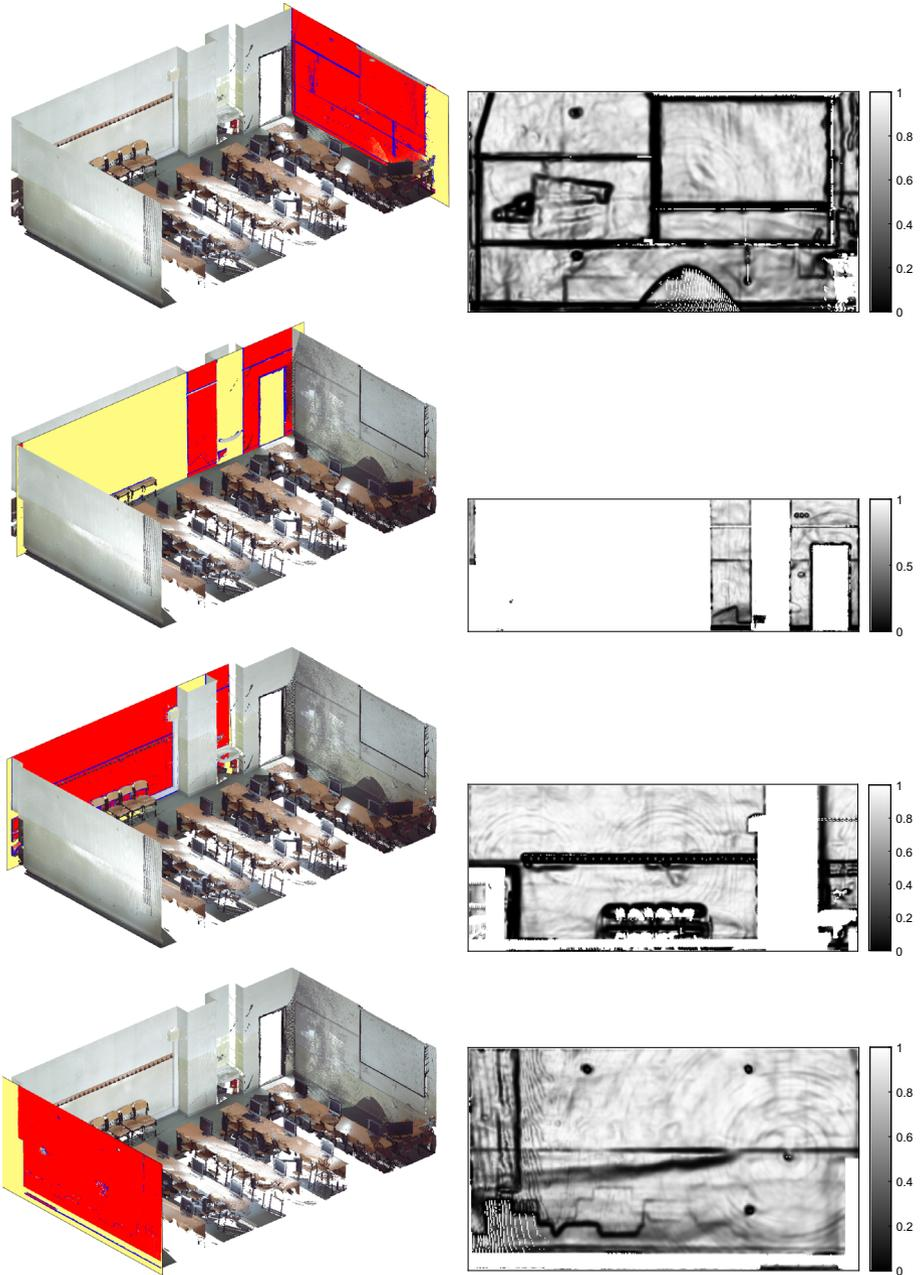
**Fig. 21** Left column: primary segmentation of the point cloud. Red points belong to the resulting planar point clouds and the blue points were rejected by the normal filter. Right column: corresponding smoothed edge detector functions
