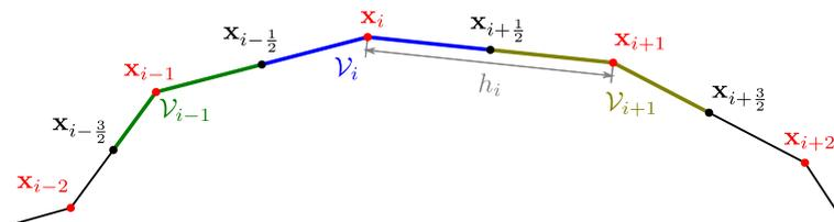
Fig. 11 The notation on the curve mesh
