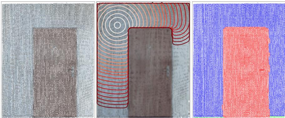
(a) The planar point cloud. (b) Beginning of the curve segmentation. (c) Segments of the point cloud.
