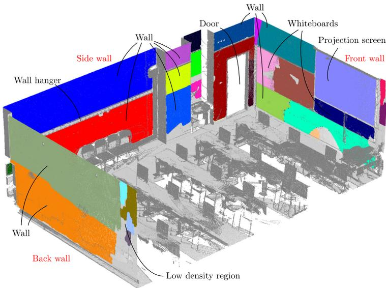
**Fig. 22** Final segments of the point cloud after segmentation of the largest walls
