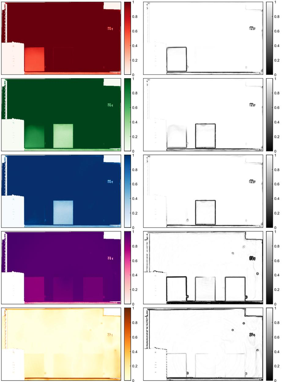
**Fig. 8** Left column: Bitmap images  $T^l, l = 1, \dots, 5$  generated from the channels R, G, B, I, D of the point cloud. Right column: corresponding edge detector functions  $g^l, l = 1, \dots, 5$
