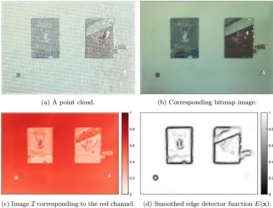
**Fig. 5** Construction of the smoothed edge detector function for the red channel
