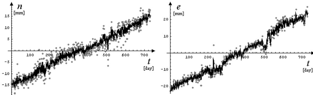
Figure 13: Visualized fit of the built model. Original data are represented by dotted, model by joined plot of a) north and b) east component.
